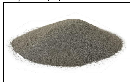
Figure2. Iron Powder about 100 mesh (about 150 \mu\text{m} )
