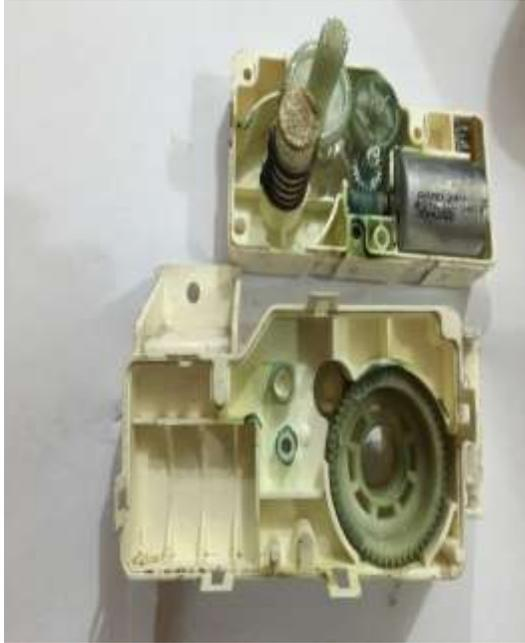
Fig( 5) DC motor with gearbox
