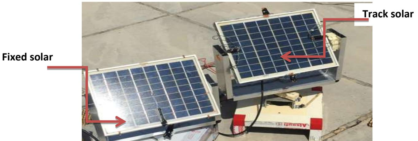
Fig(12) Comparison between fixed and track solar systems.
